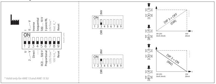
The actuator has a selection of DIP switches under the removable cover.
