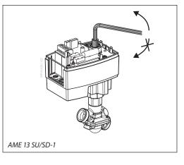
On spring versions manual override is achieved by disconnecting the power supply, removing the cover and inserting a 6 mm Allen key (not supplied) for AME 13 SU/SD-1, into the top of the positioning spindle and turning the key against the spring. Observe the direction of rotation symbol. To hold a manual override position, the key must be wedged.
