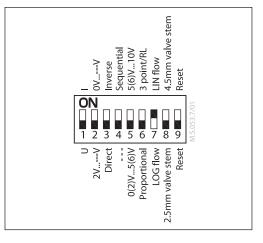
The actuator has a function selection DIP switch under the removable cover.
