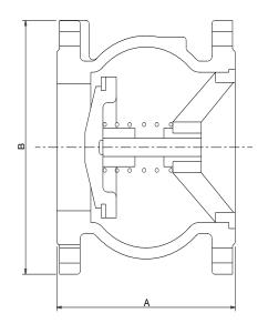
PRESSURE / TEMPERATURE RATING: 16 bar from -10 to 110°C (WRAS to 85°C) SPECIFICATION: Flanged to BS EN 1092-2 PN16.
